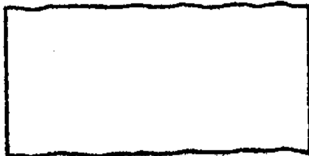
Good SSB Signal Pure Tone Input
