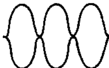
SSB WITH CARRIER, TONE INPUT IMPROPER AMPLIFIER BIAS
