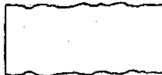
SSB Signal, Tone Input Poor Sideband Suppression
