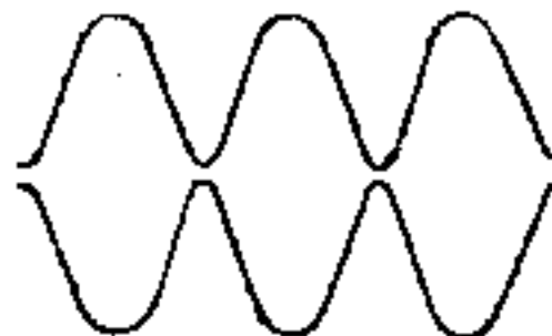
DOUBLE SIDEBAND AM WITH CARRIER 100% MODULATED
